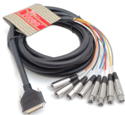
Figure 4-7: An example of a DB25-to-XLR breakout cable (sold separately) for 8-channel AES/EBU input and output. This cable has four female XLR connectors and four male XLR connectors. See Appendix D, “DB25 to XLR Pin Outs” page (109) for pin out details.
