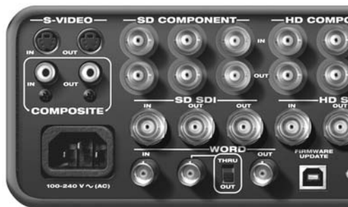
Figure 4-10: Audio word clock connectors.
