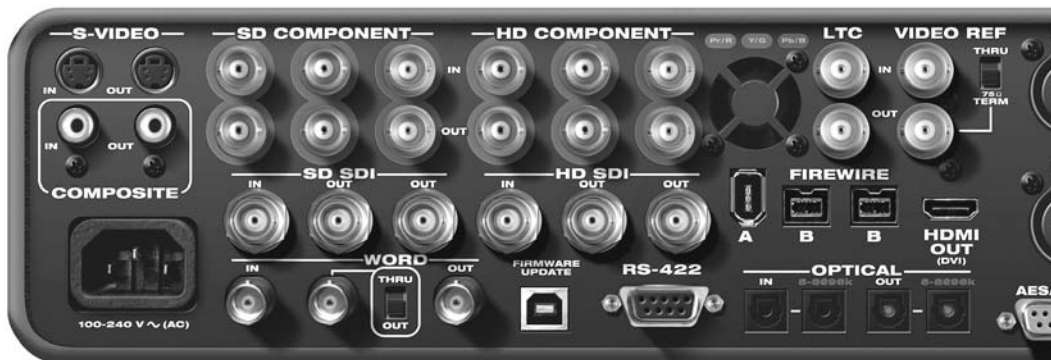
Figure 4-2: The V4HD video connectors.
