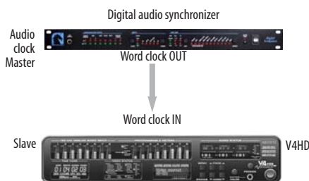
Figure 4-11: Slaving the V4HD to word clock. For the V4HD clock source, choose ‘Word Clock In’. This configuration is only supported when the V4HD is running in Audio Only mode (video features are disabled).
