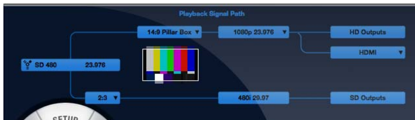
Figure 7-13: An example of hardware conversion during playback. Premiere Pro is playing back 480p23.976. The V4HD hardware is simultaneously inserting 2:3 pull-down for SD playback and converting to 1080p23.976 with 14:9 pillar box formatting for HD playback.
