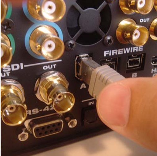
Figure 4-1: Connecting the V4HD to the computer.
