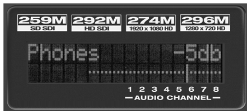
Figure 12-4: For many settings, the LCD “zooms in” on the setting as you adjust it.
