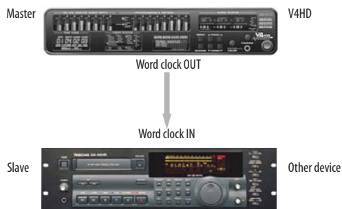
Figure 4-12: Slaving another digital audio device to the V4HD via word clock. For the V4HD clock source, choose 'Video Clock' or, if the V4HD is in Audio Only mode, any other clock source besides word clock.
