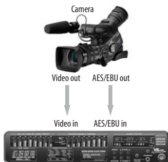
Figure 4-16: When capturing digital audio from the current video source, the V4HD genlocks to the source input, which keeps the digital audio clock properly resolved to the video source audio clock.
